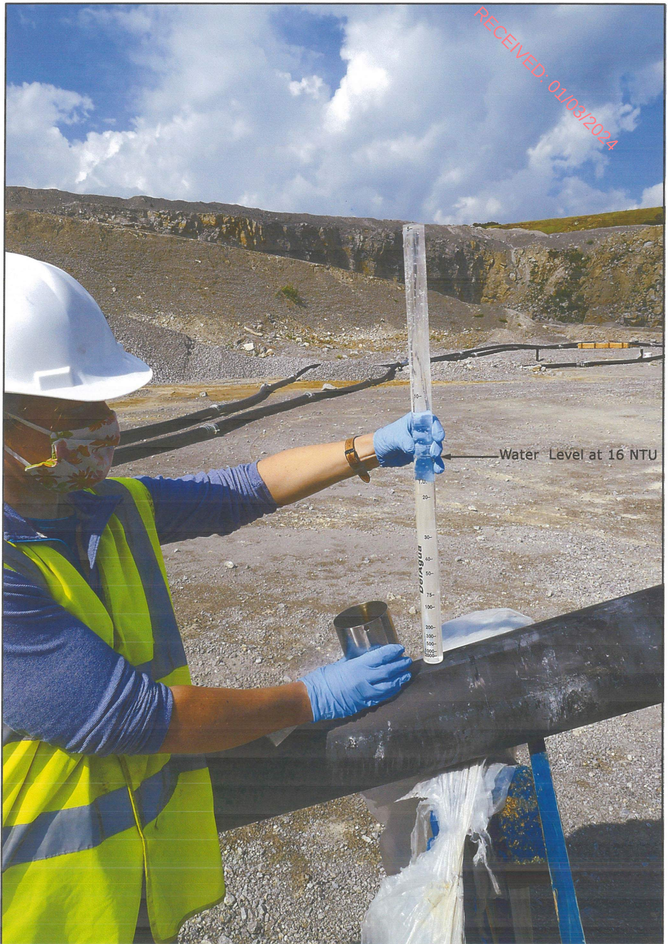
Field use of the Palintest (Del Agua) Turbidity tube in the Rathcore quarry to monitor the turbidity of water from the test boreholes before pumping to the settlement pond
