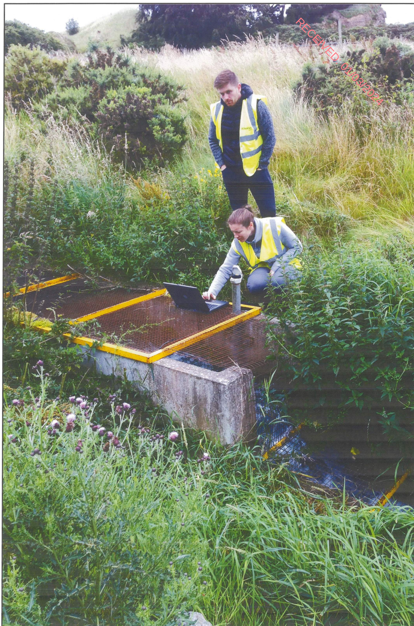
Figure 3.6 Downloading data from Ott flow meter in 'V' notch weir chamber
